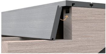
6. Snap the Riser board into place and fix it with a face screw. (Position screw correctly to be hidden by board fastened to next tread)
