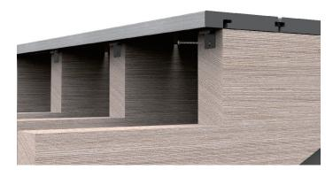
5. Install the starting clips at the top of the vertical face of the joist.
